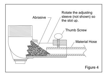
**5.2.5** When the correct mixture is achieved, tighten the thumb screw only enough to prevent movement, and rotate the sleeve so the holes are facing upward.
